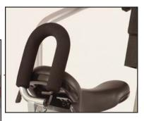
The rear stop behind the seat can be adjusted in depth. First lift up the rear stop and tilt it backwards. This reveals an Allen screw inside the Uprofile When the Allen screw is loosened, the rear stop can be slid forwards or backwards in the external tube. After adjustment, re-tighten the Allen screw.
