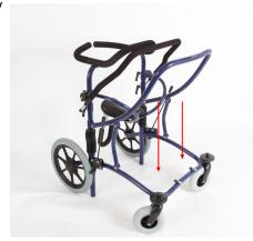
The brakes are parking brakes which function by directly blocking the rear wheels with a fitting which presses against the tire. To brake the walking aid, pull the brake levers all the way back until they come to a definite stop. In this position the brakes are self-locking. The brakes are released by pushing the brake levers forward again.
