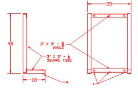
\* REAR 3 - HEX BOLTS 3/8 X 3.5 WITH 2 1/2 LAG SHIELD (DRILL 5/8 HOLE) \*\* FRONT: 2 - HEX BOLTS 5/16 X 2.5 WITH 1 3/4 LAG SHIELD (DRILL 1/2 HOLE) ALL HARDWARE ONCLUDED WITH FLOOR FRANE
